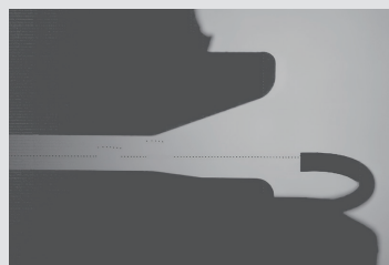
Ink drop flight evaluation with a high-speed camera
